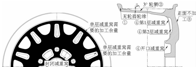
图 12 优化前车轮背腔的减重窝结构 Fig.12 Weight-decrement cavity of back cavity before optimization
